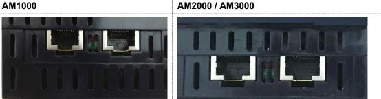
• LED green: On if a network connection (link) exists, flashes during communication
