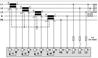
If current  $I_{\ensuremath{\mathsf{N}}}$  does not need to be measured, the corresponding transformer can be omitted. If voltage  $U_{\mbox{\scriptsize NE}}$  does not need to be measured, connection of PE can be omitted.
