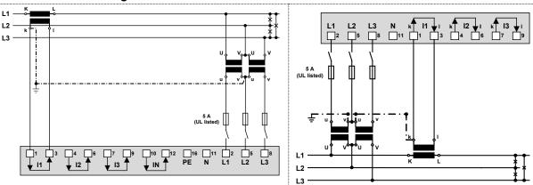
In case of current measurement via L2 or L3 connect the device according to the following table:
