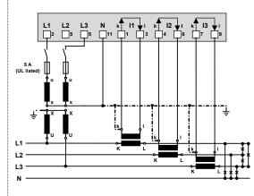
If current  $I_{\ensuremath{N}}$  does not need to be measured, the corresponding transformer can be omitted. IN is not available for the AM2000.
