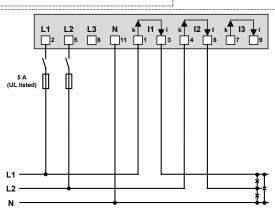
If current I<sub>N</sub> or voltage U<sub>NE</sub> does not need to be measured, connection of IN or PE can be omitted
