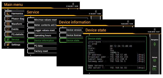
Depending on the settings of the DHCP server the provided IP address can change on each reboot of the device. Thus it's recommended to use the DHCP mode during commissioning only.
