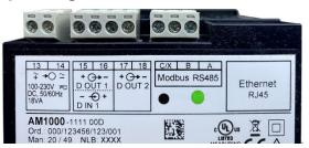
The operating LED of the AM1000 without display shows the present device state.
