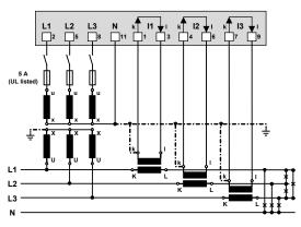
If current  $\mathsf{I}_N$  does not need to be measured, the corresponding transformer can be omitted. IN is not available for the AM2000.
