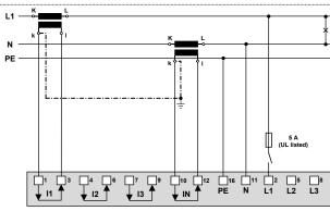
If current  $I_{\rm N}$  does not need to be measured, the corresponding transformer can be omitted. If voltage  $U_{\rm NE}$  does not need to be measured, connection of PE can be omitted.
