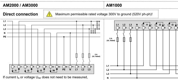
connection of IN or PE can be omitted.
