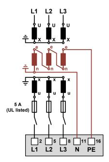
In order for the homopolar voltage to be measured, the item "Measure homopolar voltage" must be set to "Yes" in the settings of the measurement. This item is only available for 3-wire system types. Single-phase AC mains
