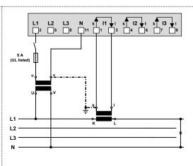
If voltage  $U_{NE}$  does not need to be measured, the corresponding transformer can be omitted. PE is not available for AM2000.
