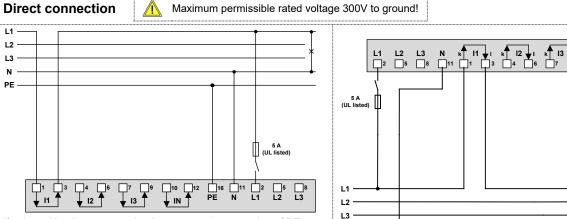
If voltage  $U_{NE}$  does not need to be measured, connection of PE can be omitted. PE is not available for AM2000.
