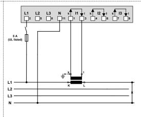
If voltage  $U_{NE}$  does not need to be measured, connection of PE can be omitted. PE is not available for AM2000.
