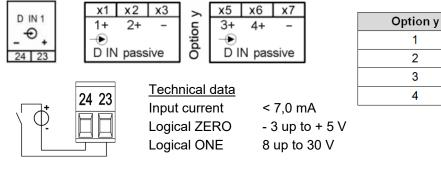
Active inputs (no external power supply required)
