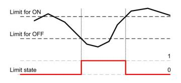
Using limit values either the exceeding of a given value (upper limit) or the fall below a given value (lower limit) is monitored.
