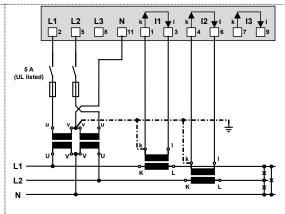
If current I<sub>N</sub> does not need to be measured, the corresponding transformer can be omitted. IN is not available for the AM2000. In systems without a primary neutral conductor a voltage transformer with a secondary center tap can also be used.
