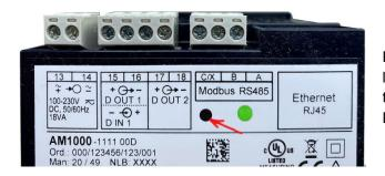
Press the sunk-in reset button (located on the left of the operating LED) for at least 3s. For that the nameplate needs to be penetrated. During the reset the operating LED flashes red.
