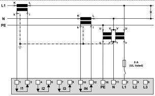
If current  $I_{\text{N}}$  or voltage  $U_{\text{NE}}$  does not need to be measured, the corresponding transformers can be omitted.
