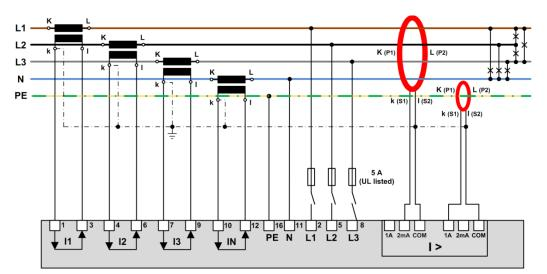
Example: Fault current monitoring in a TNS system Hint: The connections IN and PE of the device are available for the AM3000 only.
