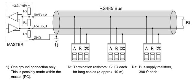
The signal wires (A, B) have to be twisted. GND (C/X) can be connected via a wire or via the cable screen. In disturbed environments shielded cables must be used. Supply resistors (Rs) have to be present in bus master (PC) interface. Stubs should be avoided when connecting the devices. A pure line network is ideal.
